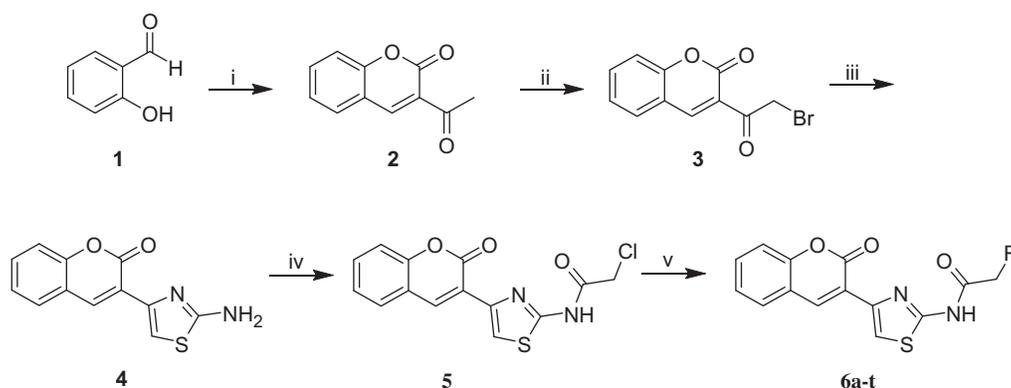
**Scheme 1.** Synthesis of new coumarylthiazole-substituted acetamide derivatives. Reaction conditions: (i) Ethylacetoacetate, piperidin, rt, 30 min; (ii) Br<sub>2</sub>, CHCl<sub>3</sub>, 50 °C, 15 min; (iii) Thiourea, EtOH, 80 °C, 2 h; (iv) Chloroacetylchloride, Et<sub>3</sub>N, THF, 70 °C, 8 h; (v) RNH<sub>2</sub>, DMF, 60 °C, 12 h.
