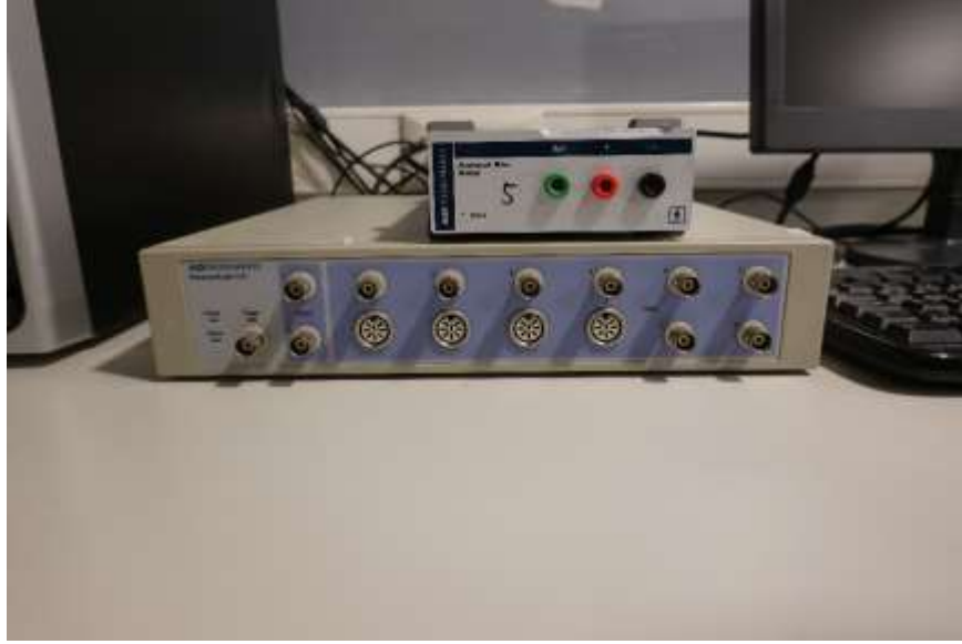
Şekil 3.3: Bioamplifikatör (ADInstruments Japan Inc. TowaTakaoka Building 2-28-24 Izumi Higashi-Ku Nagoya 461-0001 JAPAN).
