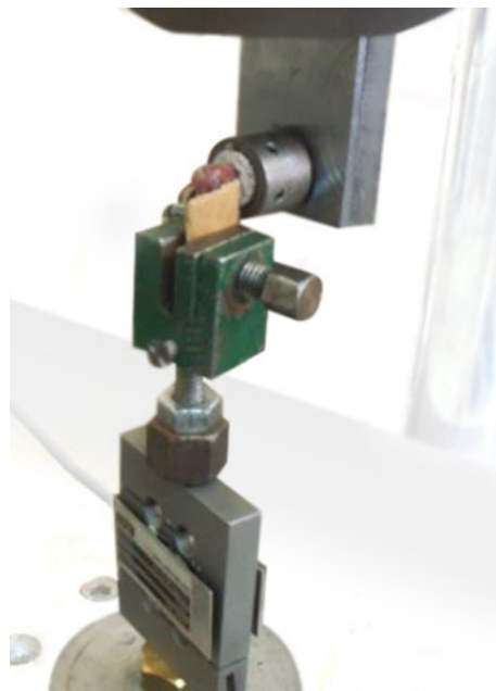
Fig. 4 Biomechanical testing set-up
