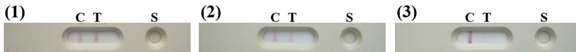
Figure 4. Test strip cassettes showing red-colored test line and control line following application of a strong and weak positive sample (1 and 2) and only red-colored control line following application of a negative sample (3). C represents control line; T, test line; S, sample application window.
