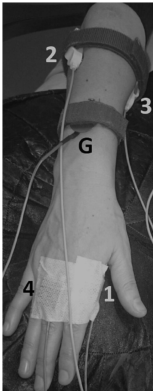
Fig. 1. Electrode/Sensor placement. Channel 1: Accelerometer sensor attached on the extensor surface of the 3rd finger metacarpophalangeal joint, channel 2: Surface EMG electrode pair placed on the forearm extensor muscles, channel 3: Surface EMG electrode pair placed on the forearm flexor muscles, channel 4: Accelerometer sensor attached on the lateral surface of the 2nd finger metacarpophalangeal joint, G: Ground.
