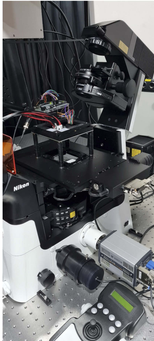
Fig. 5. Picture of our Fourier ptychography microscope with fluorescence imaging capability.
