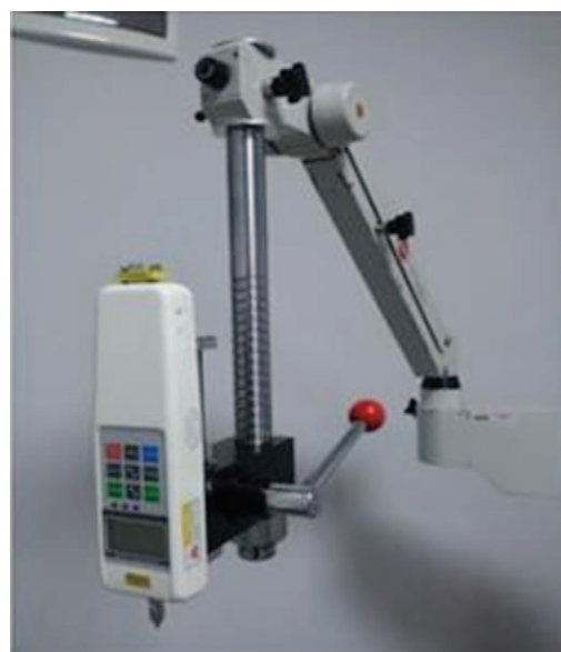
FIGURE 2. Sundoo SH-10 Digital Dynamometer assembled to Sundoo SPJ stand.
