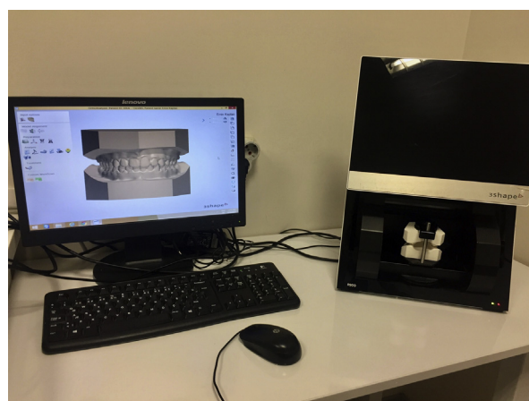
Fig 1. Three-dimensional scanning of dental casts with 3Shape R900 scanner.
