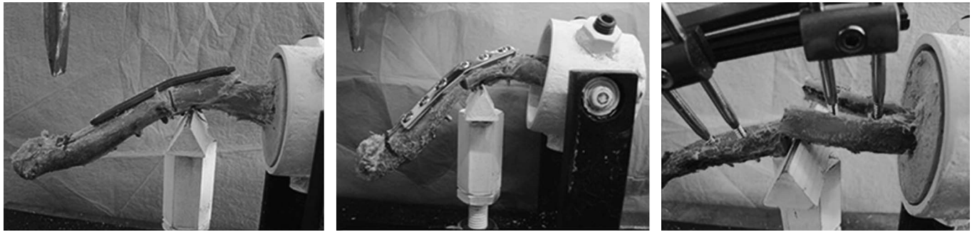
FIGURE 4. Failure modes (bending tests).
