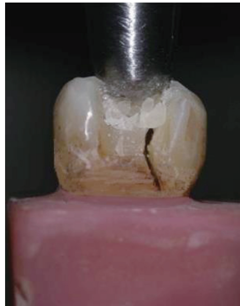
Fig. 2 Positioning and axial compressive loading of specimen in universal testing machine.
