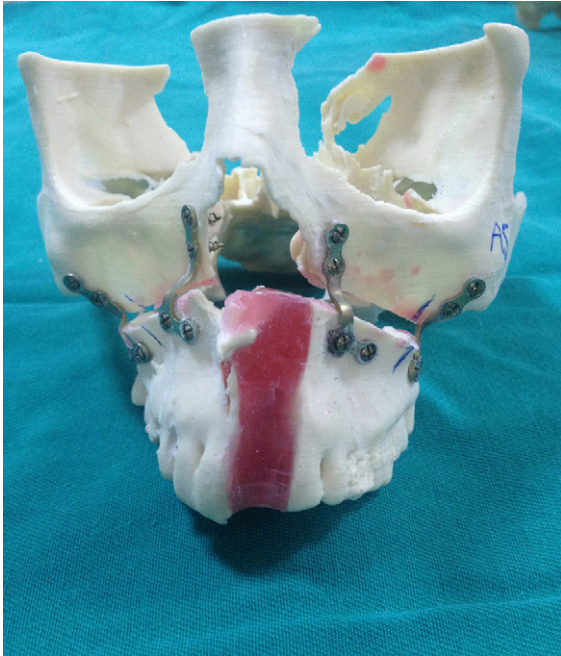
Fig. 1. Standard titanium L-shaped miniplates 1 mm thick and 2.0 mm diameter screws adapted and placed bilaterally ( 2 \times 1 mm group).
