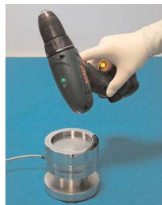
**Fig. 4.** Microbiological sampling from the venting ports of the electric drill. [Color figure can be viewed in the online issue, which is available at [www.aott.org.tr](http://www.aott.org.tr)]
