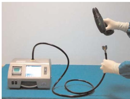
**Fig. 3.** Particle counting from the venting ports of the electric drill. [Color figure can be viewed in the online issue, which is available at [www.aott.org.tr](http://www.aott.org.tr)]
